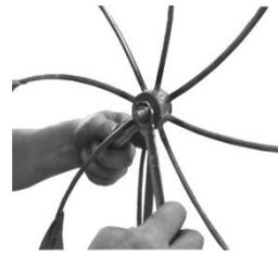
Tighten P4 snugly and then loosen so that there is about a 1/16 inch give.
