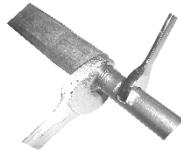
2. Hold "B" into place with an 11/16" wrench and tighten "A" (turning clockwise) with the 7/16" wrench (you may use 2 adjustable wrenches instead)
